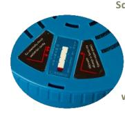
Squeeze the bubble on the rear of the TIS strip until it flattens. Remove the cover from its adhesive band, locate the outer end in the slot in the recess and firmly press into place as shown. The red line will creep along the window over time.
