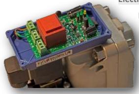
Low power consumption with operating indicators Local full test circuit to check and exercise system Intelligent control measures rate of discharge Closes valve before escape of compressed air Local alarm indication + contacts for remote alarm
